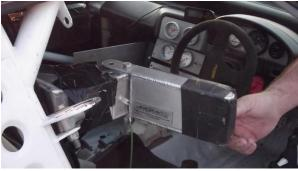
Below is an example of a NON COMPLANT Lateral Helmet restraint,
