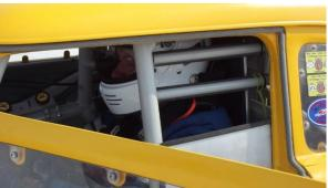
NOTE: The restraint must extend to the forward most portion of the helmet as shown above.
