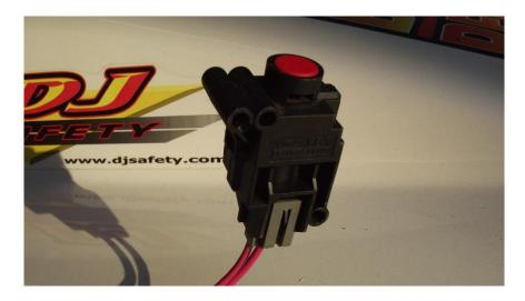
NOTE: If you are running a mechanical fuel pump, it is advisable (NOT a rule) to still have an INERTIA switch, but on the ignition circuit.
