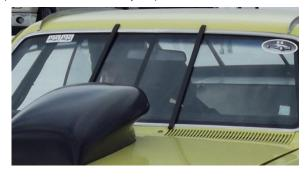
IF your vehicle has polycarbonate (Lexan) windscreens, you may be permitted to run without window tabs/straps, provided the windows are mounted SECURELY! (An example in below photo).
