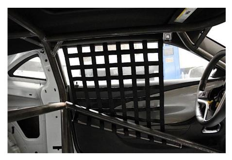
The net/restraint above does not comply at all. It is outside the roll structure, and the front edge will not protect the driver's hand/wrist. Also, the restraint does not cover the entire door area. As per, there is no net or panelling below the intrusion bar.
